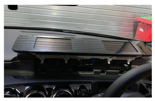
THE SCREEN WILL JUST LIFT UP ONCE YOU HAVE REMOVED THE 2 X T20 SCREWS, THIS WILL THEN GIVE YOU ACCESS TO THE REAR OF THE SCREEN
