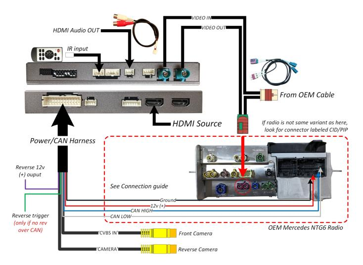
**NOTE** : Manual gearbox vehicles may require green wire trigger for reverse switching.
