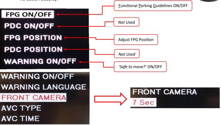
To activate *Front Camera timer*, scroll down using the remote arrow keys when in the menu to *FRONT CAMERA*. Once in this setting, press OK and choose (up/down) between 5, 7, 9 or 11 seconds for *auto-front switching timeout* (once the vehicle leaves reverse gear, the front camera input will stay active for pre-defined amount of time).
