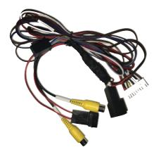
CONNECT THE POWER / CAN HARNESS AT THE HEAD UNIT. Installation
