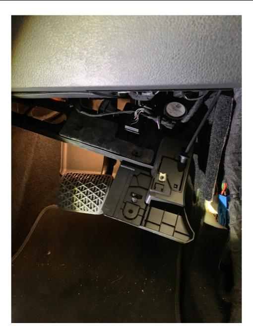
The radio tuner is typically located high in the passengers kick panel area, or underneath the seat. You will need to access the main power connector for ground (-), 12v (+) constant, CAN HIGH and CAN LOW.
