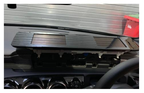
THE SCREEN WILL JUST LIFT UP ONCE YOU HAVE REMOVED THE 2 X T20 SCREWS, THIS WILL THEN GIVE YOU ACCESS TO THE REAR OF THE SCREEN
