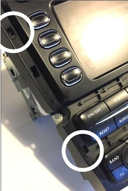
**Remove the 4 x trim clip from original ZAB unit and clip into the supplied fascia**
