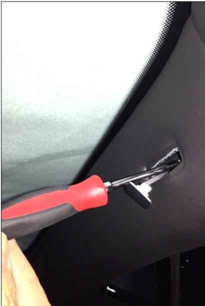
**For the after market microphone and possible DAB antenna (GT / SPUR: N/A for US vehicles) remove the A pillar trim**
