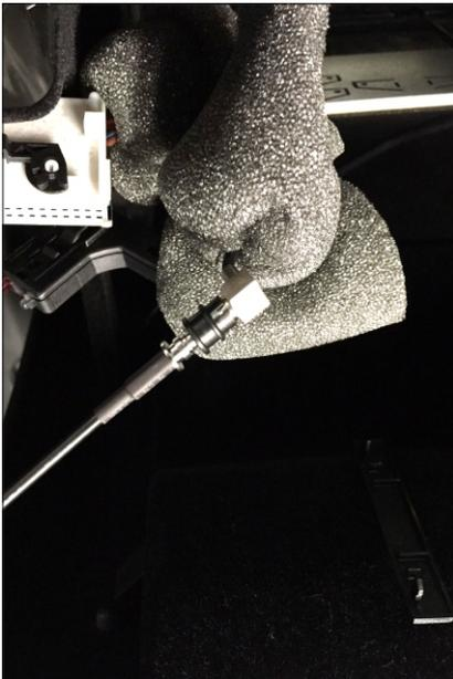
Connect the supplied GPS extension lead to the OEM GPS socket behind the CD navigation drive
