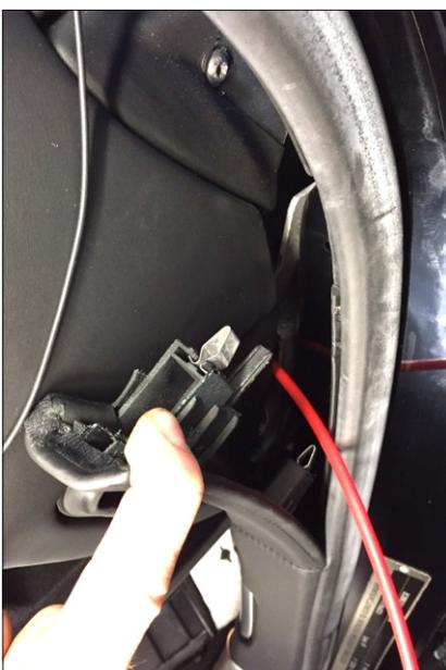
**Pry back trim next to door seal and use a feeder cable to get through to the glove box**
