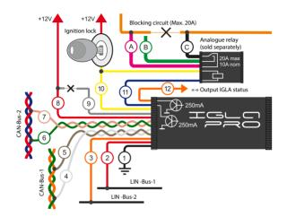
Connection to LIN-1 and LIN-2 makes it possible to use the digital LIN-bus for **disabling the start of engine**. In this case it is not necessary to connect analogue relay for blocking. Use the analogue relay (sold separately) to enable the function **stall of the running engine**, see p.6 (or to enable the function engine start inhibit if there is no LIN-bus).
