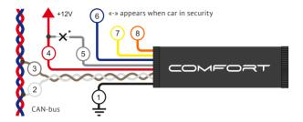
To connect COMFORT module, connect its wires in the following way:
