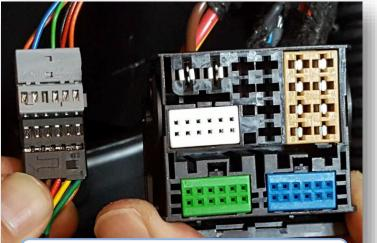
Connect OEM 12-pin to provided 12-pin (black, PIN-side). *NOTE: printed arrow location on provided 12-pin plug vs OEM plug.*
