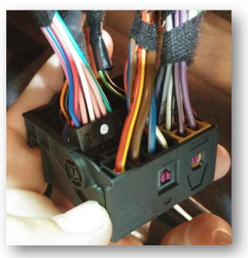
7. Connect ground and power for your camera, you may use the provided brown wire (labeled 'REAR12VOUT') for power for convenience. NOTE: This power source will only supply 12v when the vehicle is in reverse (if forced rear camera is desired at any time, you'll need to use an ACC source for power instead).
