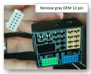
Connect the female 12-pin side of the plug & play portion to the OEM main MIB connector as shown. *Note the paint dot must face towards the thick power wires.*
