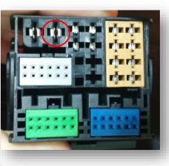
6. Connect the provided 12-pin plug & play portion from the main power harness to the main factory MIB radio connector as shown below. Pay attention to the orientation, as this is vital to proper operation:
