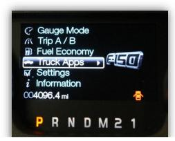
Using the steering wheel controls scroll down to the *Truck Apps* function in the instrument cluster.
