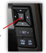
3. Press the "OK" button on the steering wheel.
