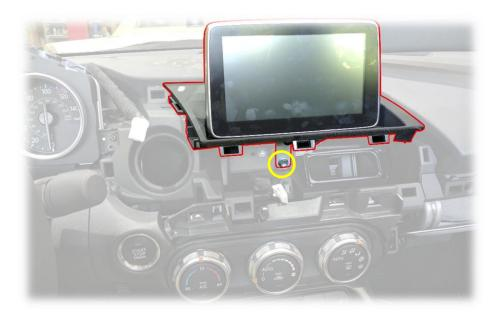
The two plugs to be tied into for this install are circled below. The S2P module included in this kit is required to power on the camera when the door is unlocked (unlocking the door wakes the CAN-BUS, thus powering the camera so that it is ready when the vehicle is started). If the S2P is *not installed*, the camera displaying while in reverse gear will be *intermittent*.
