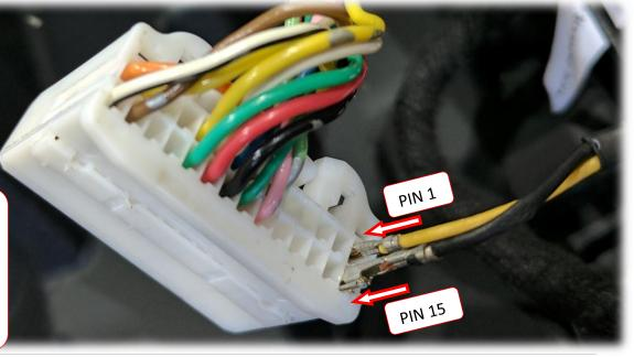
Press the pin-lock tab down on the same connector (from step 8) to secure the pins into the connector.
