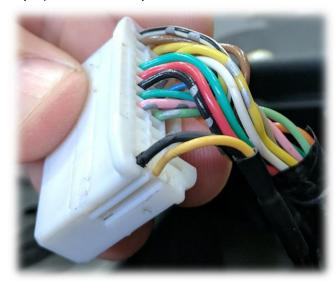
This step is vital for reliable camera operation for this install. Ground the camera power to a chassis ground (-) or splice to the same ground on the S2P power harness.
