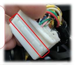
**8.c.** Insert the RCA shield (black) pin into PIN 15 and the RCA signal (yellow or clear) into PIN 1.
