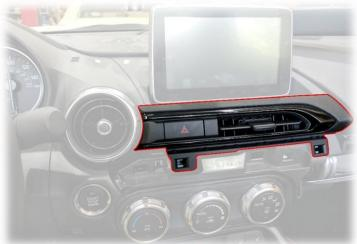
3. Next, pull the cluster shroud (with vents) out towards you. They are secured to the sub-dash with clips only. Disconnect the sensor harness and set this panel aside.
