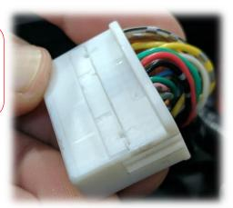
**8.b.** With a pick tool, pry open the pin-lock tab NOTE: the tab does not fully remove!
