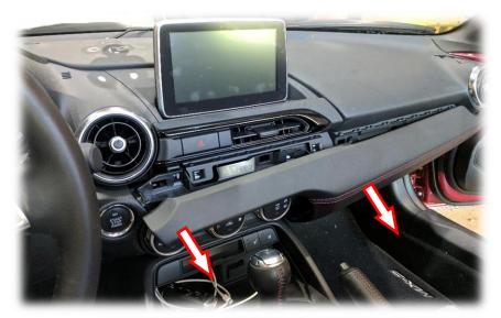
2. Next, pull the vent assembly with hazard switch out towards you. It is secured to the sub-dash with clips only. Disconnect the hazard switch.
