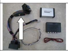
6. If your vehicle is not equipped with a stock camera and you are not installing a front camera then simply unplug the male RCA end from the female in the aftermarket harness and run your camera's video RCA directly to the female plug. Connect ground for the reverse camera to the black wire and 12 volt positive to the white/red from step 5 and insulate the white/blue wire. Skip to step 8
