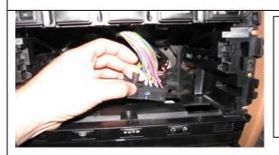
8. Plug the fiber optic cable you unplugged in step 3 into the aftermarket harness. Reconnect all the antenna, power and all other connectors back into the radio and slide the radio back into the dash. Reassemble in the reverse order as steps 1,2 and 5. Now you are ready to proceed to the programming and operations section. Good job!
