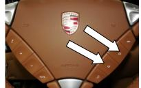
When SERVICE is displayed on the screen, press and hold the up arrow for 4 seconds to program the PCM for reverse camera.
