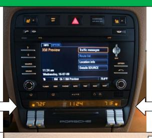
1. Insert a soft pry tool into the space between the lower black fascia piece and the lower side of the dash and gently pry the fascia towards the rear of the vehicle to release the mounting clips. Follow the fascia around either clockwise or counterclockwise to release the remainder of the mounting clips. Set aside the fascia.
