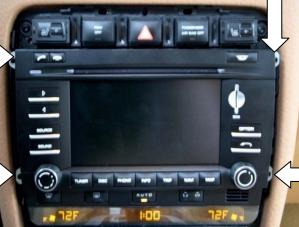
2. Remove (4) t20 torx screws from the sides of the radio and pull the radio gently out of the dash in order to disconnect all stock cables and antenna connectors.
