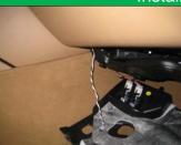
5. Drop the plastic panel over the passenger side kick panel area by taking out (1) t20 Torx screw and pulling the panel towards the floor. Run the black, white/blue and white/red wires from the new radio harness into the opening as in the picture to your left. These wires will power your reverse and front cameras, as well as the video switcher.
