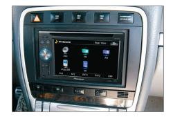
Place facia plate on the dashboard. Fix it with the 4 original screws.
