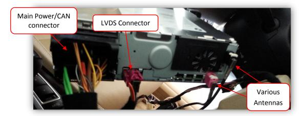
6. The main 44-pin connector at this radio is where the Power (+), Ground (-) and *twisted* CAN wires must be connected. From the BMW12 interface POWER/CAN plug, connect the following:
