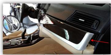
2. Disconnect all harness connected to this panel (near the vents mostly). You may want to remove the push button ignition switch so that you can test the BMW12 interface prior to replacing the dash panels. Either unclip this assembly or remove (3x) Torx screws and then reconnect to the vehicle plug:
