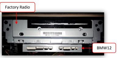
10. Connect the provided *LVDS video cable* to the factory BMW screen. Run the other end of the LVDS behind the vents and connect it to the BMW12 interface at the port labeled 'LCD-OUT'.
