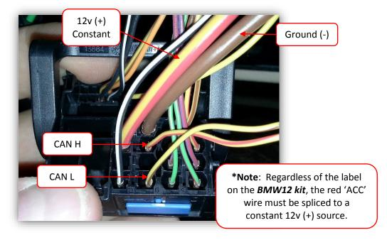
7. After making the power/CAN connections, you must replace the factory LVDS video cable with the LVDS cable provided in the BMW12 kit. To access this plug (behind the factory LCD screen), remove (2x) Torx screws:
