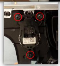
Remove (2x) Torx screws securing the radio controls and climate control face, pry outwards and disconnect all harnesses:
