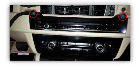
4. You should now see the disc-player portion of the radio. Remove this assembly be removing (2x) more Torx screws:
