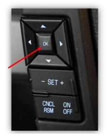
3. Press the "OK" button on the steering wheel.
