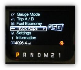
Using the steering wheel controls scroll down to the *Truck Apps* function in the instrument cluster.
