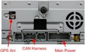
7. Connect a 10' pair of wires to the ALLSync module. Connect one of the wires to pin 6 and the other to pin 16. Route the free end of the wire pair through the firewall (at your incision), into the engine bay of the vehicle. Use silicon or 3M strip caulk to seal the incision.
