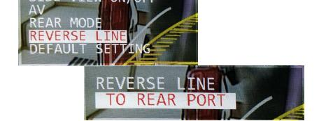
To set custom *green wire trigger*, find 'REVERSE LINE' option and set to 'REAR PORT' or 'AV1' depending upon your preference. Every time the green wire receives 12v (+), the selected RCA port will display on screen.
