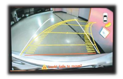
Press and hold the *back arrow* on the steering wheel to cycle the screen from OEM image, to HDMI (if adapter was added), to connected front camera (if no change, try check Dip Switches 1 & 2 and your menu settings). Otherwise, the front camera will display (whenever you leave the *reverse gear*) for the user-set amount of time (5, 7, 9 seconds, etc).
